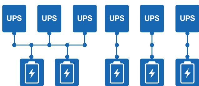
3 frames in parallel with Common Battery
