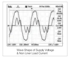
The main contributor to this is the nature of load current drawn by these equipments. These equipments, to remain more power efficient, uses regular power waveform in a "chopped" manner. In the process, they become "non-linear" type of load, a load is said to be non-linear when the current it draws does not have the same wave form as the supply voltage.
