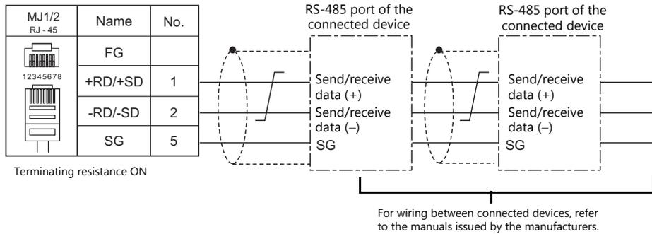
\* Set the slide switch for signal level selection to RS-232C/485 position (upper) when using the MJ2 port of V907W or V906.
