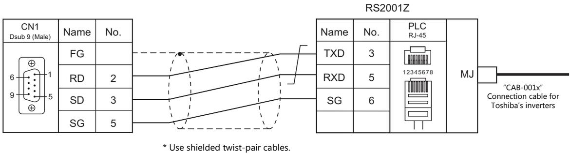
Wiring diagram 2 - C2
