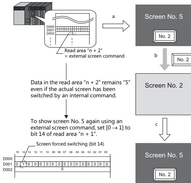
Reset this bit (OFF) after checking that bit 14 of write area "n + 1" is ON, or the value stored in write area "n + 2" is the same as the value in read area "n + 2".
