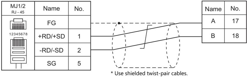
**Wiring diagram 5 - M4**
