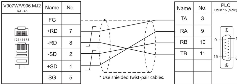
\* Slide switch on V907W/V906:
