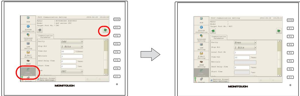
4. Configure [Local Port No.] and press the [Apply] switch.
