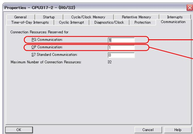
Connectable number of units when the PG protocol is selected (Including connections with STEP 7)
