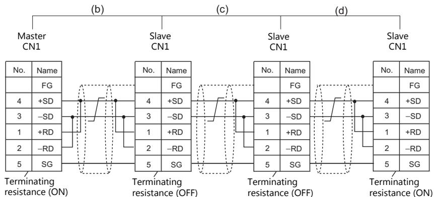
\* As a measure against noise, connect the frame ground terminal of each V9 series at one side only.
