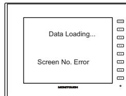
Before starting communications with the PLC, check the data in [Read Area] "n + 2" and confirm that the screen number to be displayed initially is specified.
