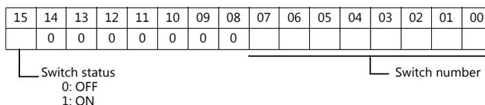
For the relationship between the switch output device memory and the switch number, see page 33-36.
