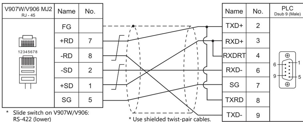
**Wiring diagram 8 - M4**
