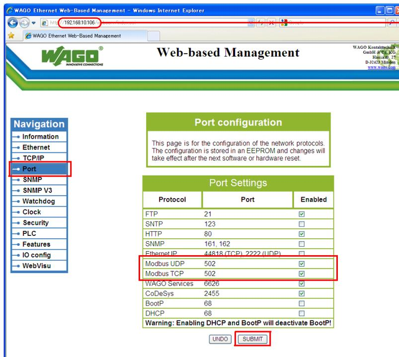
Enter the IP address of the bus coupler or bus controller on Internet Explorer, and press the [Enter] key to display the browser menu.
