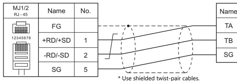
**Wiring diagram 2 - M4**
