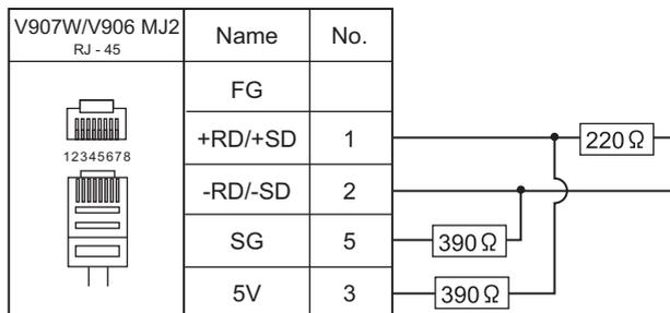
**Wiring diagram 2 - M4**
