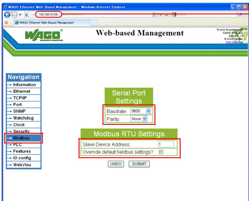
Enter the IP address of the bus coupler or bus controller on Internet Explorer, and press the [Enter] key to display the browser menu.
