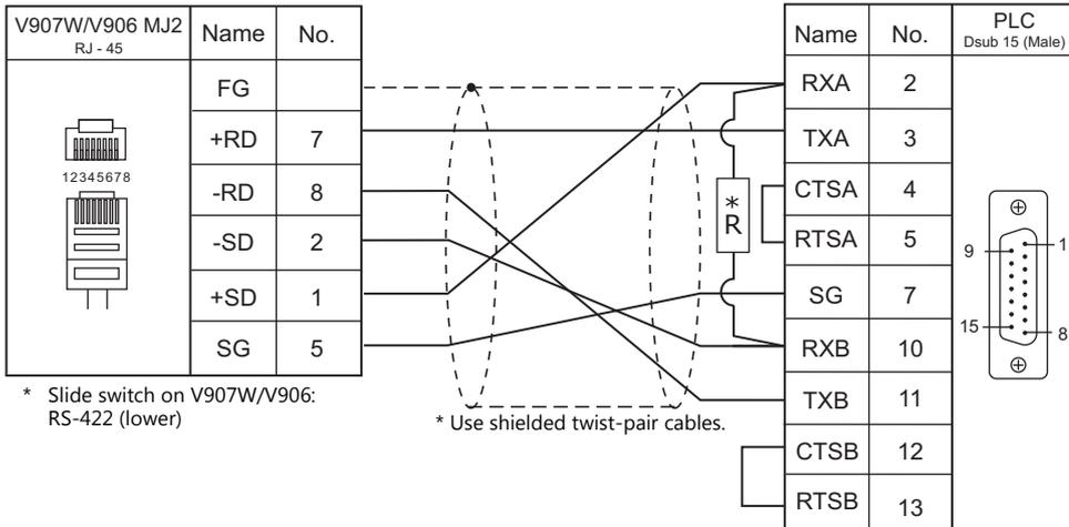
**Wiring diagram 3 - M4**
