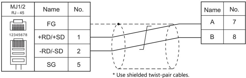
**Wiring diagram 7 - M4**
