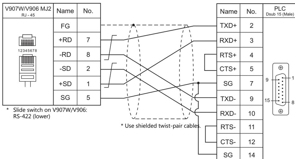
**Wiring diagram 3 - M4**
