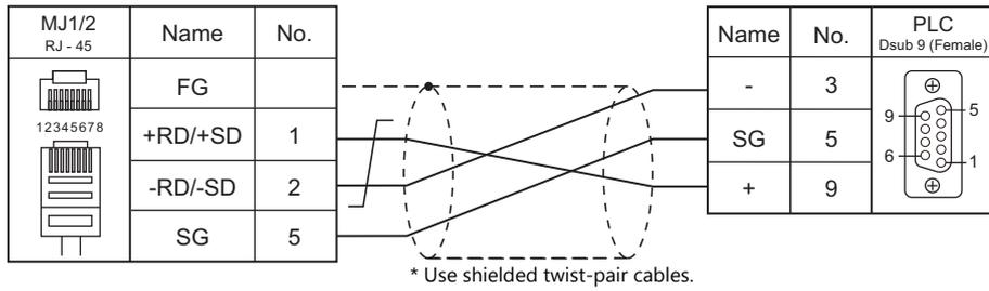
Wiring diagram 3 - M4
