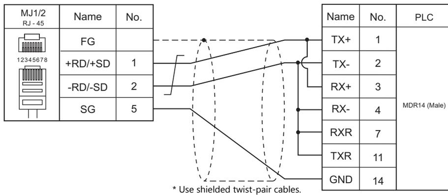
**Wiring diagram 6 - M4**
