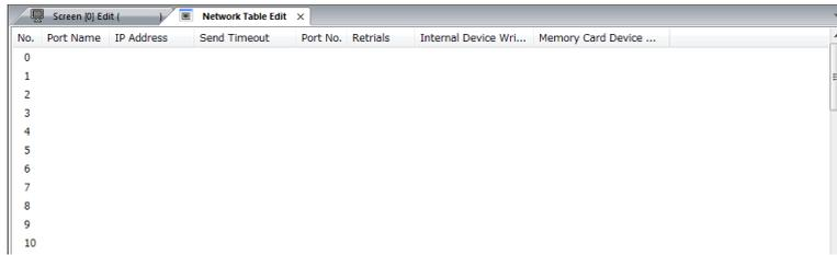
Double-click a number in the No. column to display the [Network Table Setting] dialog. An IP address and other items can be registered.
